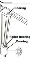
**Both doors have the unique gravity hinge (Patent Pending) featuring:**
